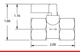
Maximum Operating Pressure — 500 psi Maximum Operating Temperature — 180°F Ball Through Hole Diameter — .312
