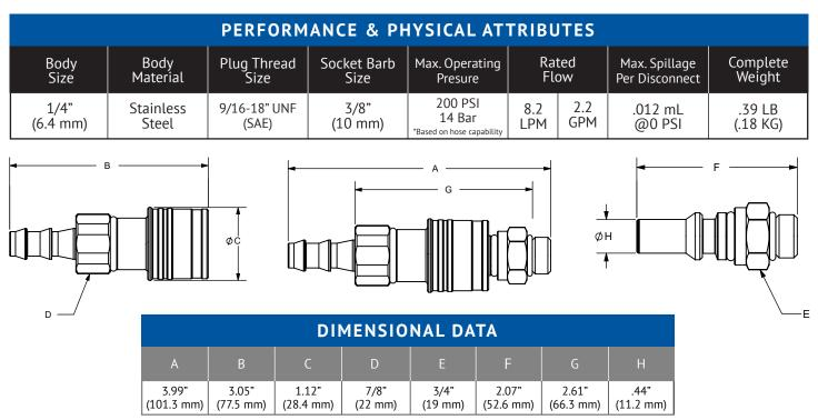
Temperature Range: Standard seals EPDM max operating temperature 150°F (65°C). Vacuum Data: 27.4 inches Hg. both connected and disconnected pressure rating (Max. Operating Pressure) is based on non-pulsating, low cycle applications with essentially steady pressure during the operating cycle. Please consult factory regarding other applications.
